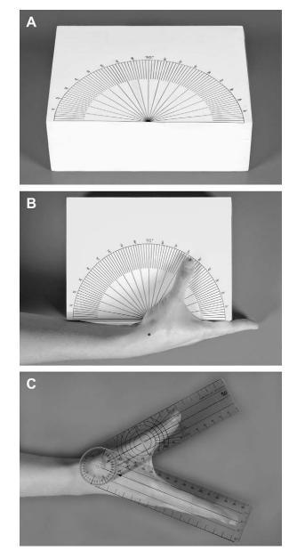
**FIGURE 1.** (A) The Pollexograph with a protractor on top. The Pollexograph has a length of 21 cm, height of 7 cm, width of 13.5 cm, and a radial protractor length of 13 cm. The protractor is divided into steps of 2°. (B) Positioning of hand and forearm with two landmarks (CMC joint and middle distal part of the nail) on the Pollexograph. (C) An active palmar abduction measurement with the goniometer placed over metacarpal 1 and metacarpal 2.
